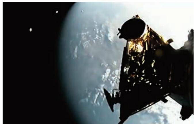
*Each Iridium NEXT satellite is secured to a dispenser ring that sits atop the second-stage rocket. At predetermined intervals, satellites are released from the ring to begin their sequenced drift into orbit.*
