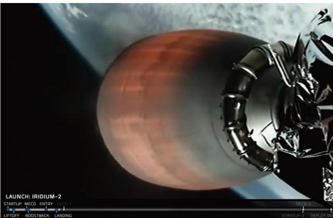
*The Falcon 9's second-stage rocket fires one engine to position the Iridium NEXT payload in the correct orbital plane. Operational satellites orbit at an altitude of approximately 483 miles above the earth.*
