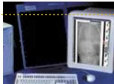
Varian's PaxScan amorphous silicon image receptors could take the place of medical X-ray film, providing instant diagnostic images, reducing patients' exposure to radiation, and eliminating the need for film processing and storage.
