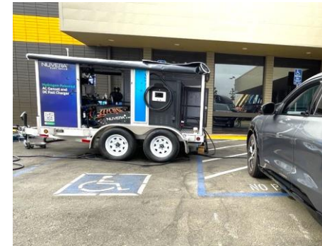
Prototype HydroCharge™ unit, a hydrogen-powered AC genset and DC fast charger for on-site power and EV charging, demonstrated at California customer site
