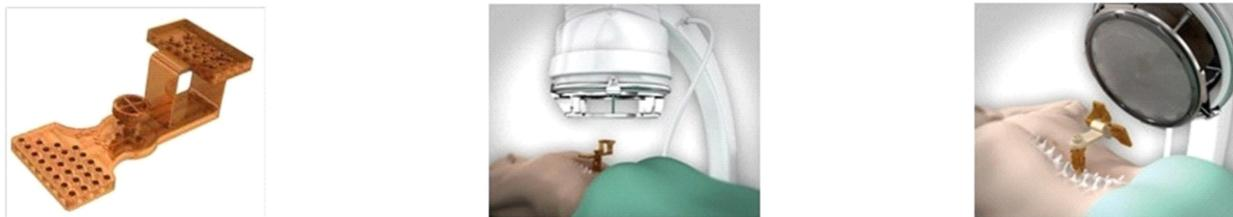
Figure 2: 3D Marker; C-arm in 2 positions taking registration images for 3D Synchronization process
