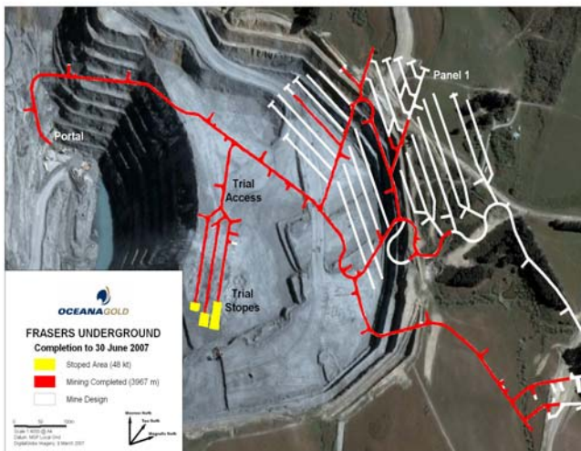
- Figure 1 - Mining completed shown in red as at 30 Jun 2007
