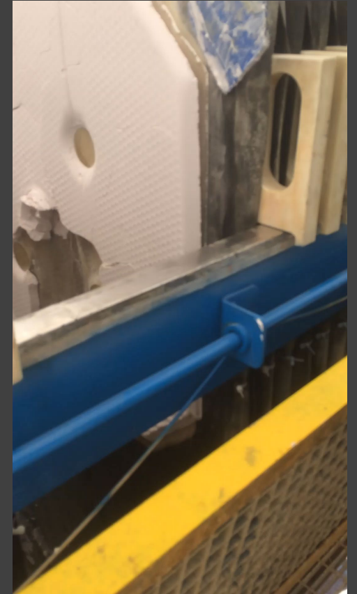
Video of 1 st mixed REE carbonate from monazite coming off of filter press at White Mesa Mill
