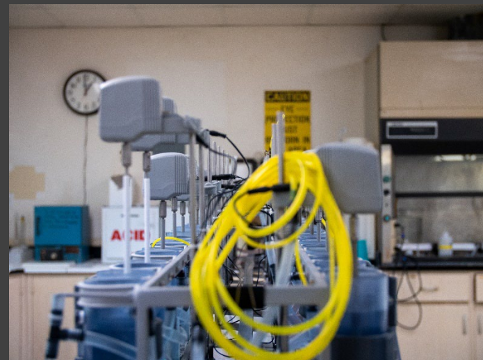
Multi-stage lab-scale solvent extraction (SX) REE separation occurring today (36-stages currently & increasing)
