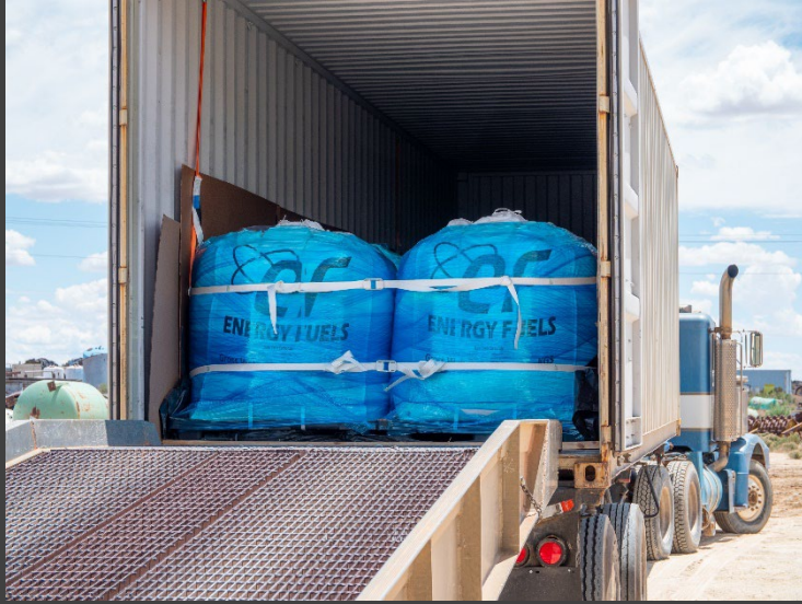
1 tonne "supersacks" of high-purity mixed RE carbonate
