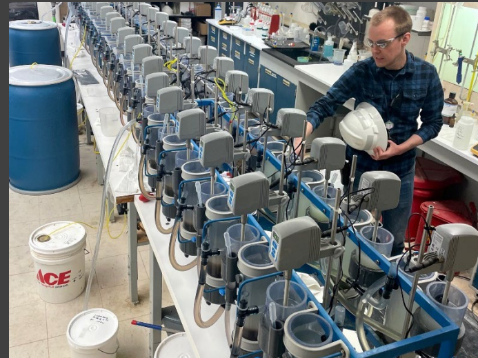
72-stage pilot-scale solvent extraction (SX) REE separation capable of producing 1-2 kg of NdPr oxide per day
