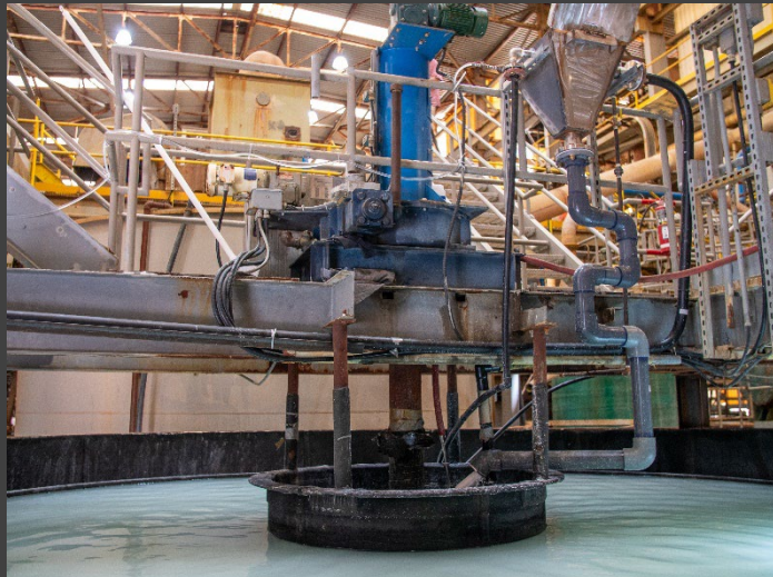
Monazite "crack-and-leach" ongoing at Energy Fuels' White Mesa Mill
