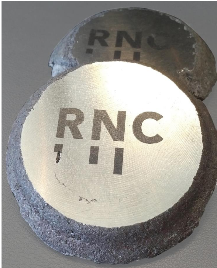
Ferro-nickel puck produced from Dumont concentrate
