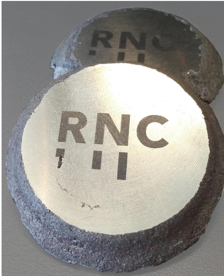
Ferro-nickel puck produced from Dumont concentrate
